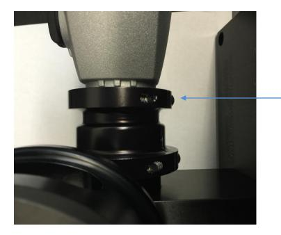
Loosen screw and then adjust electric motor to desire position and tighten screw.
