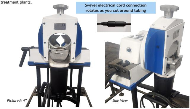
Designed to perform true and burr free cuts with our specially designed vice that creates a self-centering hold for the finest cuts.
